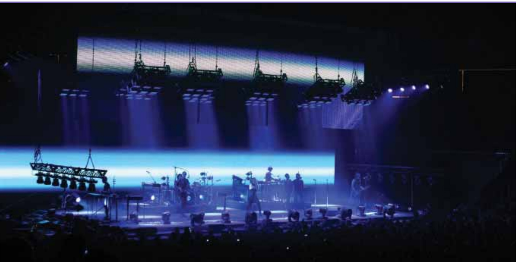
The upstage wall is a 16'-high-x-70'-wide V9 9mm wall with abstract video content from Sheridan and Moment Factory.
